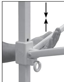
**7.** Engage the Auto Slider® at each corner by pushing up with one hand while holding down the top of the leg with the other hand. The quick pin will engage the hole. Then pull down the hem of the top. Repeat at all four corners.
