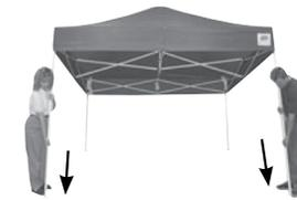
**8.** Lift two adjacent outer legs up 1" and slide out the inner legs until the toggle button locks. Repeat on the opposite legs - make sure to do two legs at a time.
