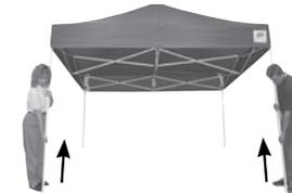
**1.** With partner, slightly lift up two adjacent outer legs 1", depress toggle button and telescope inner legs into outer legs. Repeat on the opposite legs - making sure to do two legs at a time.
